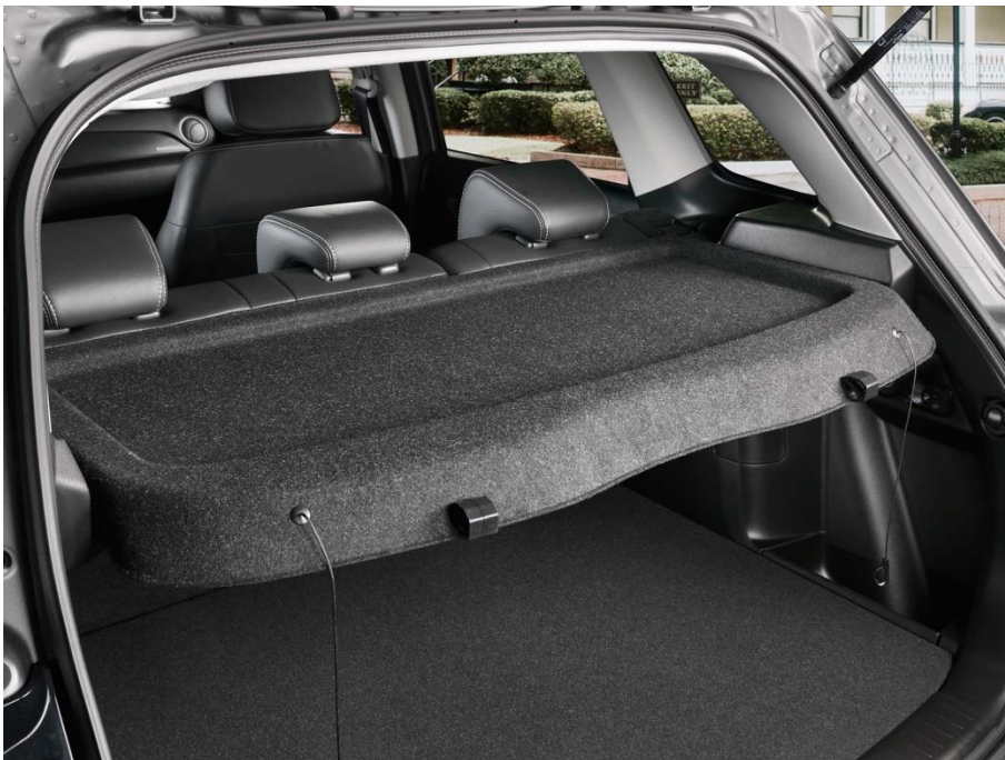
Suzuki Vitara Hutablage aus RENOLIT TECNOGOR . (Foto: RENOLIT COMPOSITES , PR001)
